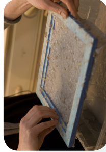
STEP 6 Drain pulp with screen
